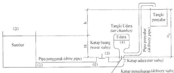
**Gambar 1.** Instalasi pompa hydraulic ram pump
